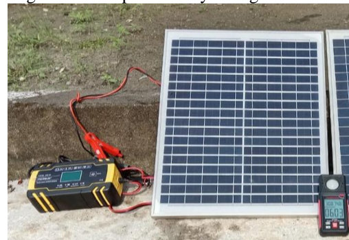
Gambar 2: Instalasi Pengukuran Panel Surya Polycrystalline
