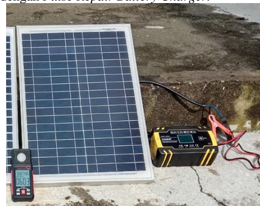
Gambar 4: Instalasi Pengukuran Panel Surya Monocrystalline
